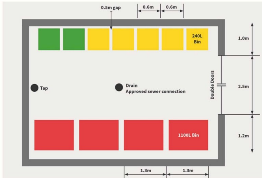
Typical bin storage room with mix of mobile bins and bulk bins
